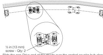
Slide the non-Drive end of the shade over the angled coupler hub closest to the drive end. Tighten the set screws in the tube adapter to secure the shade to the angled coupler hub.
