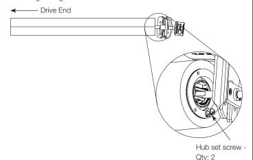
Slide the other end of the shade over the remaining hub of the first angled coupler. Tighten the setscrews in the tube adapter to secure the end of the shade to the angled coupler hub.
